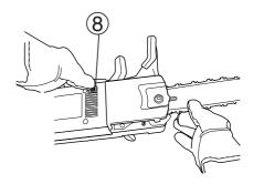
9. Tighten the mounting nut with the combination tool while holding the tip of the guide bar up.
